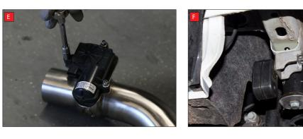
Once happy with fitment of Scorpion Exhaust, fully tighten up all clamps and fixing and plug in the electronic valve motors.
